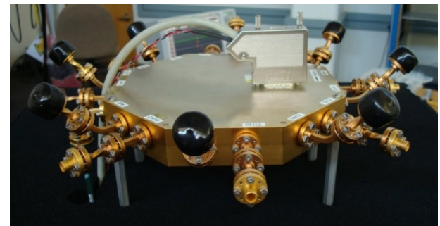
Robot-mounted array of 16 directional receive antennas
