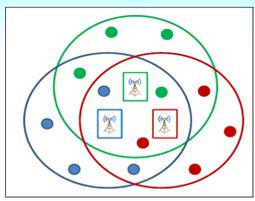
Fig. 1. System model showing an overlay deployment of three small cell clusters in a macrocell
